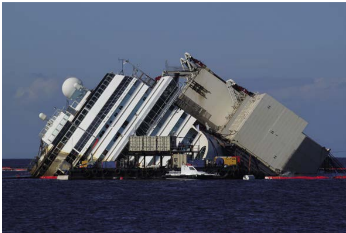
Parbuckling Concordia. (ph. credit Fagioli)
