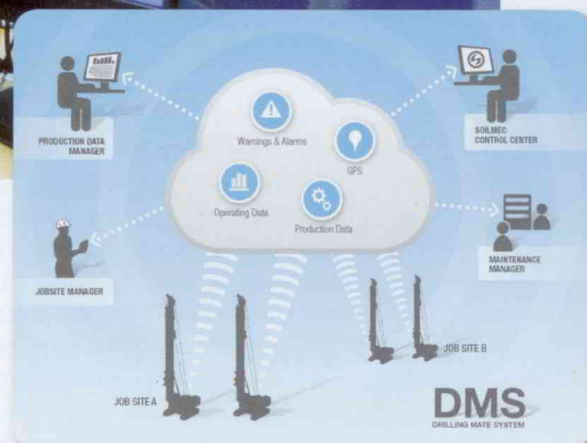
Data flow of Soilmec's Drilling Mate System. DMS allows rig operators, project managers, and Soilmec service managers to monitor machines in real time and analyze data offline.
